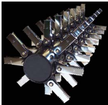
Figure 3. The new straw chopper equipped with 8 rows of knives.
